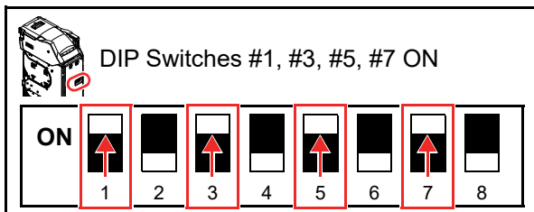
Figure 6-84 DIP Switch Test 5
